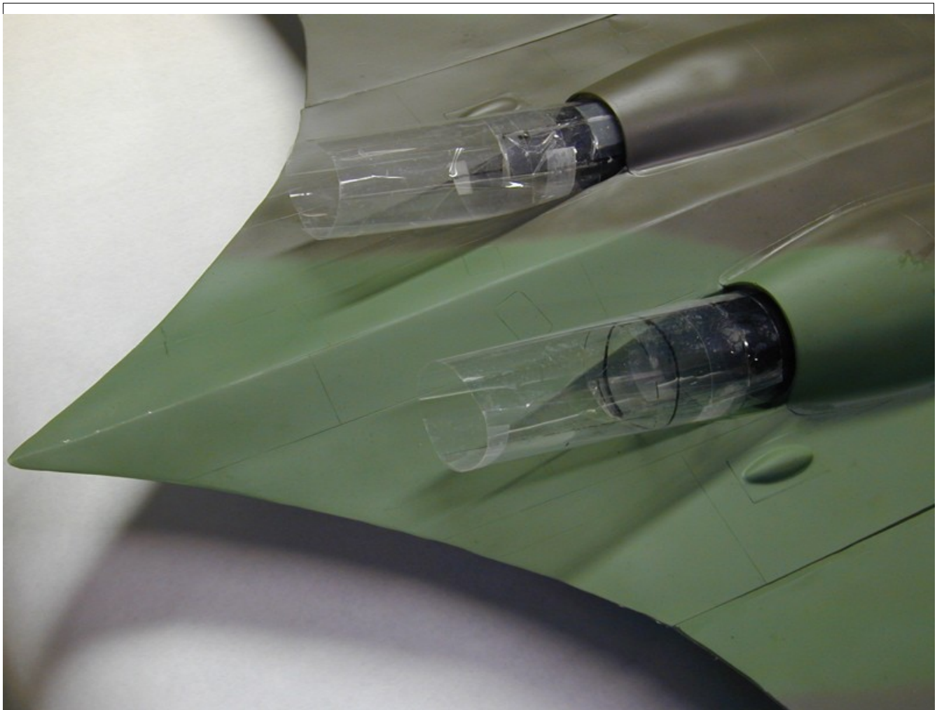
Figure 49: Exhaust extension tubes
