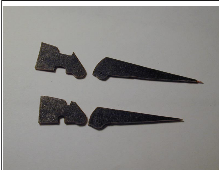
Figure 44: Flap hinges laminated with carbon fiber veil
