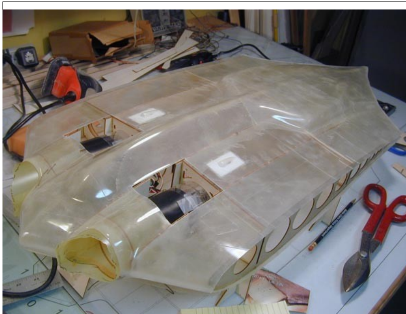
Figure 48: Lower shell attached to framework
