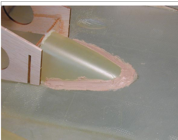
Figure 20: Rear duct fairing and filler application
