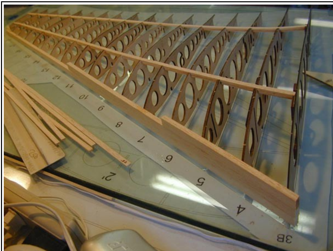
Figure 26: Leading edge installation
