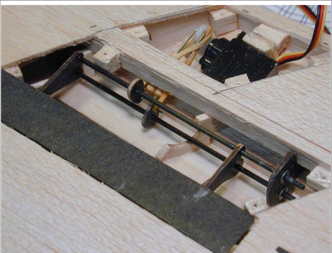
Figure 41: Completed drag rudder installation with servo and pushrods
