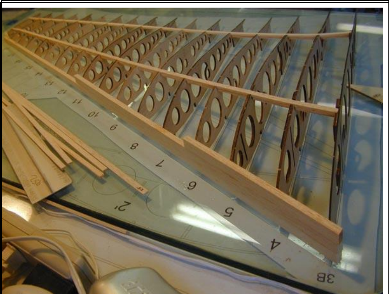
Figure 21: Leading edge installation
