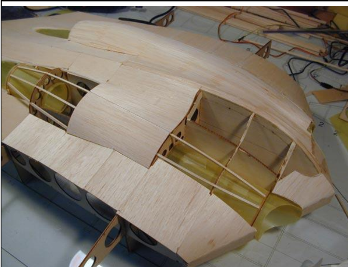
Figure 14: Preparing for Strip Planking the Engine Covers and Canopy Area
