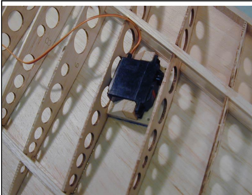
Figure 30: Elevon servo installation
