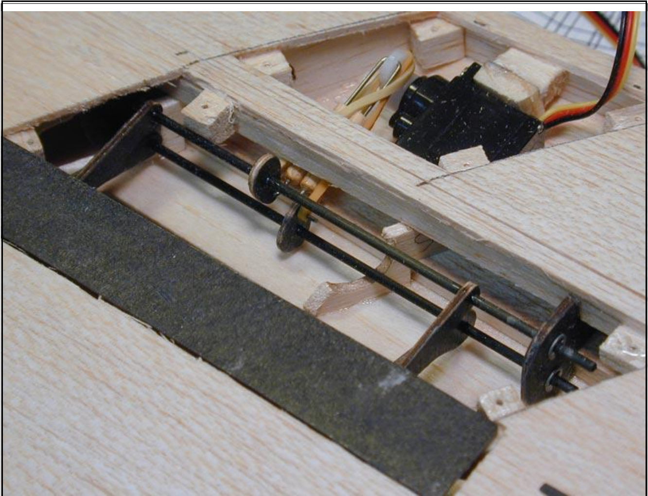
Figure 34: Completed drag rudder installation with servo and pushrods
