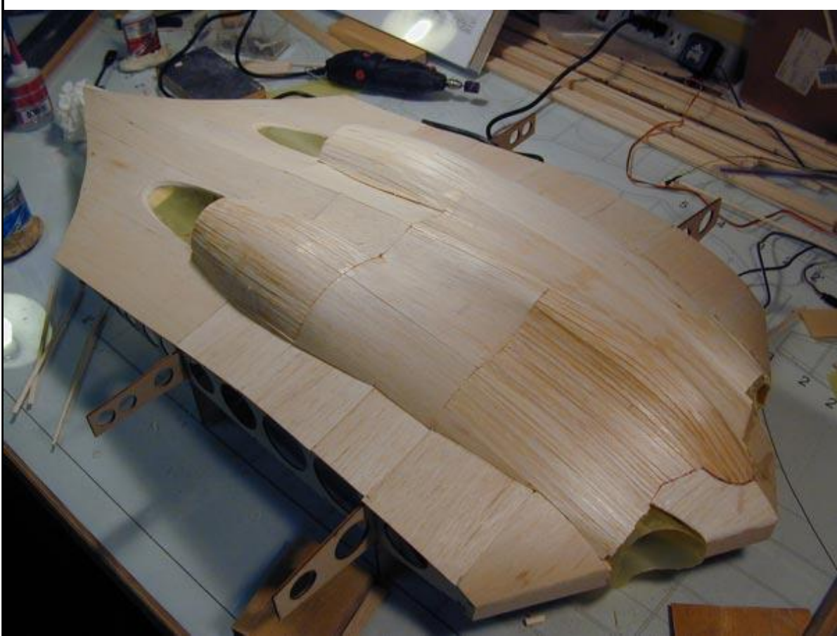
Figure 15: Finished Upper Center Section Sheeting
