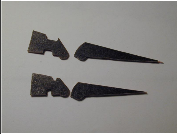
Figure 46: Flap hinges laminated with carbon fiber veil
