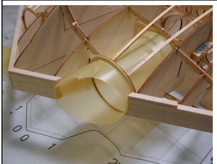
Figure 11: Intake Duct Installation
