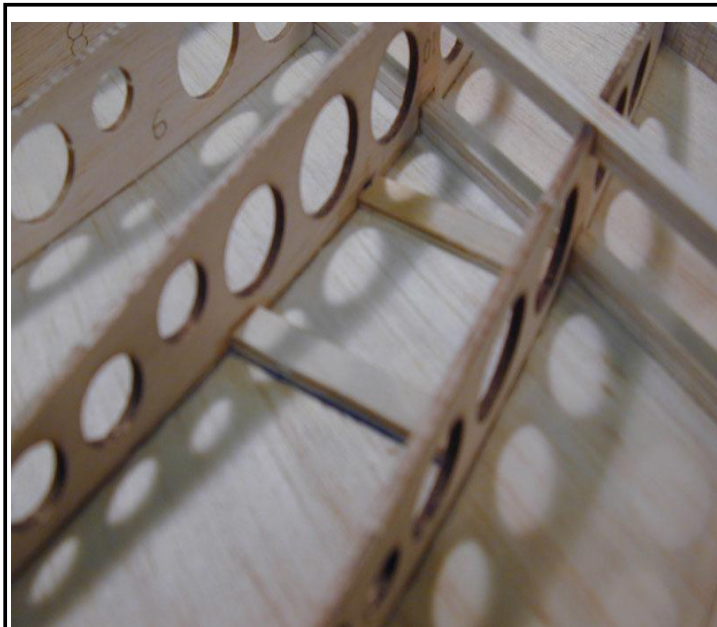
Figure 28: Installing servo rails
