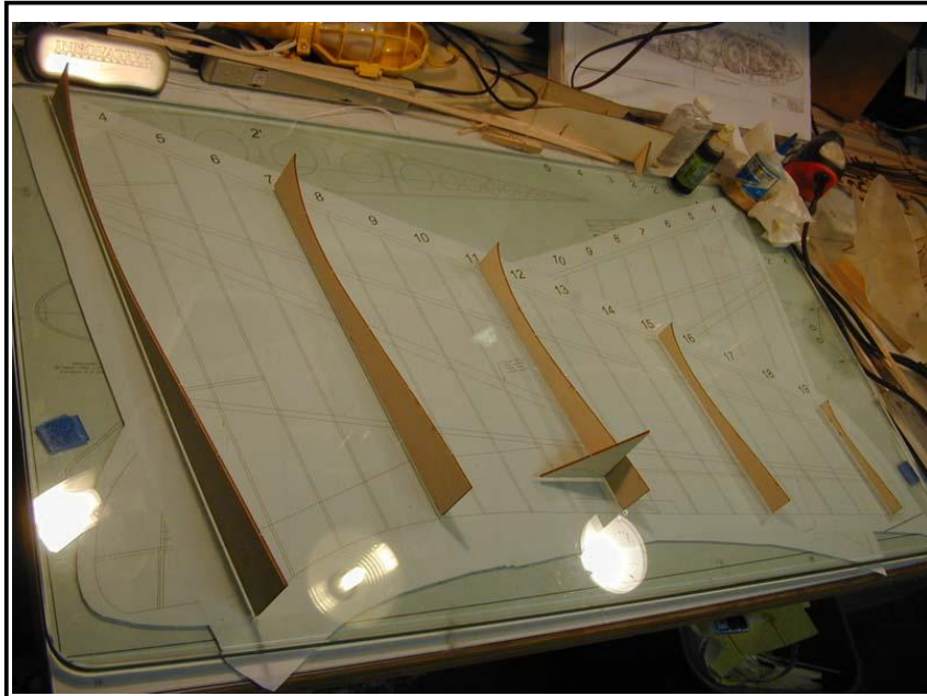
Figure 26: Attaching the wing jig to the building board
