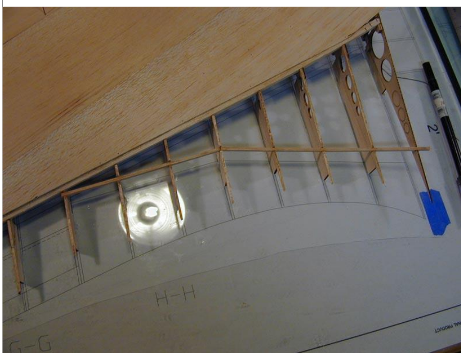
Figure 23: Upper flap sub-spar installation
