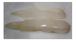
The crew nacelle is made from 5 oz glass cloth and West Systems epoxy resin. It is in two pieces, an upper and lower half. The dividing line is all on the framwork and does not cross any clear areas. Some trimming required, cut lines are scribed into the surface of the mold. The window lines are also scribed into the mold. The builder has the option of painting them on or cutting them out and using clear plastic glued to the inside.
