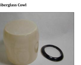
The cowl is molded in two pieces, the main cowl and a separate nose ring which can be weighted with lead shot. Plywood cowl support framework is included with laser cut parts. The cowl has scale panel lines scribed into the surface of the mold. The cowl is made from 9 oz glass cloth and West Systems epoxy resin.
